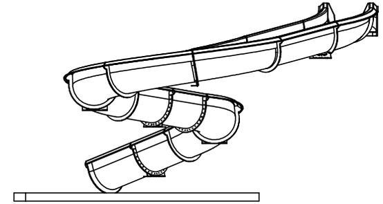
ALL 32' OPEN AND ENCLOSED FLUME SLIDES ARE CONSTRUCTED OF LAMINATED FIBERGLASS REINFORCED MARINE GELCOAT SURFACE.
