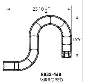
ALL 32" OPEN AND ENCLOSED FLUME SLIDES ARE CONSTRUCTED OF LAMINATED FIBERGLASS REINFORCED MARINE GELCOAT SURFACE.
