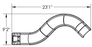
ALL 32" OPEN AND ENCLOSED FLUME SLIDES ARE CONSTRUCTED OF LAMINATED FIBERGLASS
