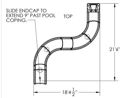
ALL 32" OPEN AND ENCLOSED FLUME SLIDES ARE CONSTRUCTED OF LAMINATED FIBERGLASS REINFORCED MARINE GELCOAT SURFACE.
